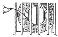
• When pumping air into tire, be sure to wear protective glasses as there is danger for dusts to get into your eye when they are blown off by compressed air.
