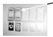
Load memory switch Push this switch for more than 2 seconds the load being handled with its value shown on display. Than, short beep is heard and stored into memory.
