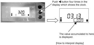
0.1P represents 100Kg on the screen. Example: 1.1P = 1.1 tons (1,100Kg)
