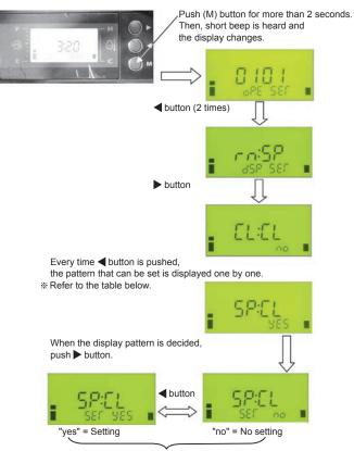
Push (M) button when the setting is completed.
