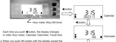
When you push (M) button with the display except the calendar, return to normal display mode. Or when once it turns off the key switch, return to normal display mode.
